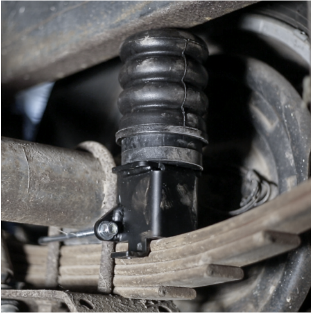
TRAILER SUMOSPRING INSTALLED
